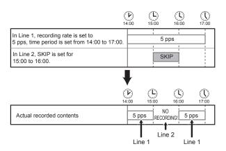
Recording is not performed correctly if there is an error in the setting. To prevent such errors for timer recording, this unit notifies errors using methods shown below. If there is an error in the setting, take the necessary procedures shown below.
